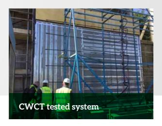
our Zinc Interlocking panel system has been CWCT tested to meet NHBC standards which can be essential on projects where there is a standard testing requirement, or alternatively functioning as a fantastic selling point providing quality assurance to your client.
